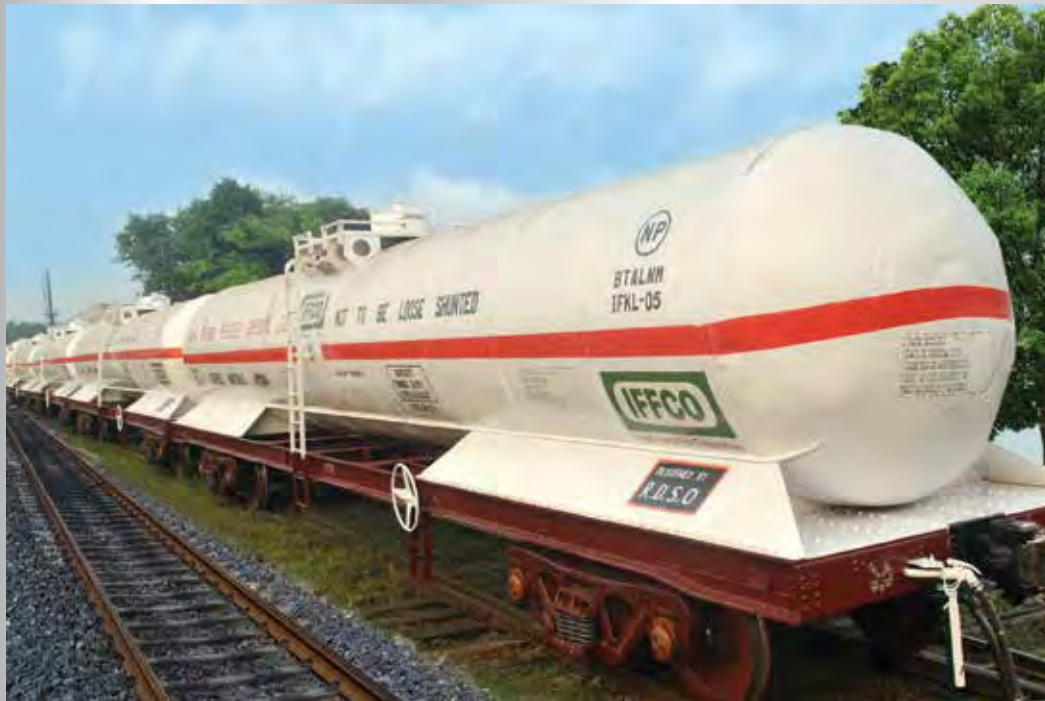
Ammonia Tank Wagon 'BTALNM' for transportation of Anhydrous Liquid Ammonia for Fertiliser Plants
