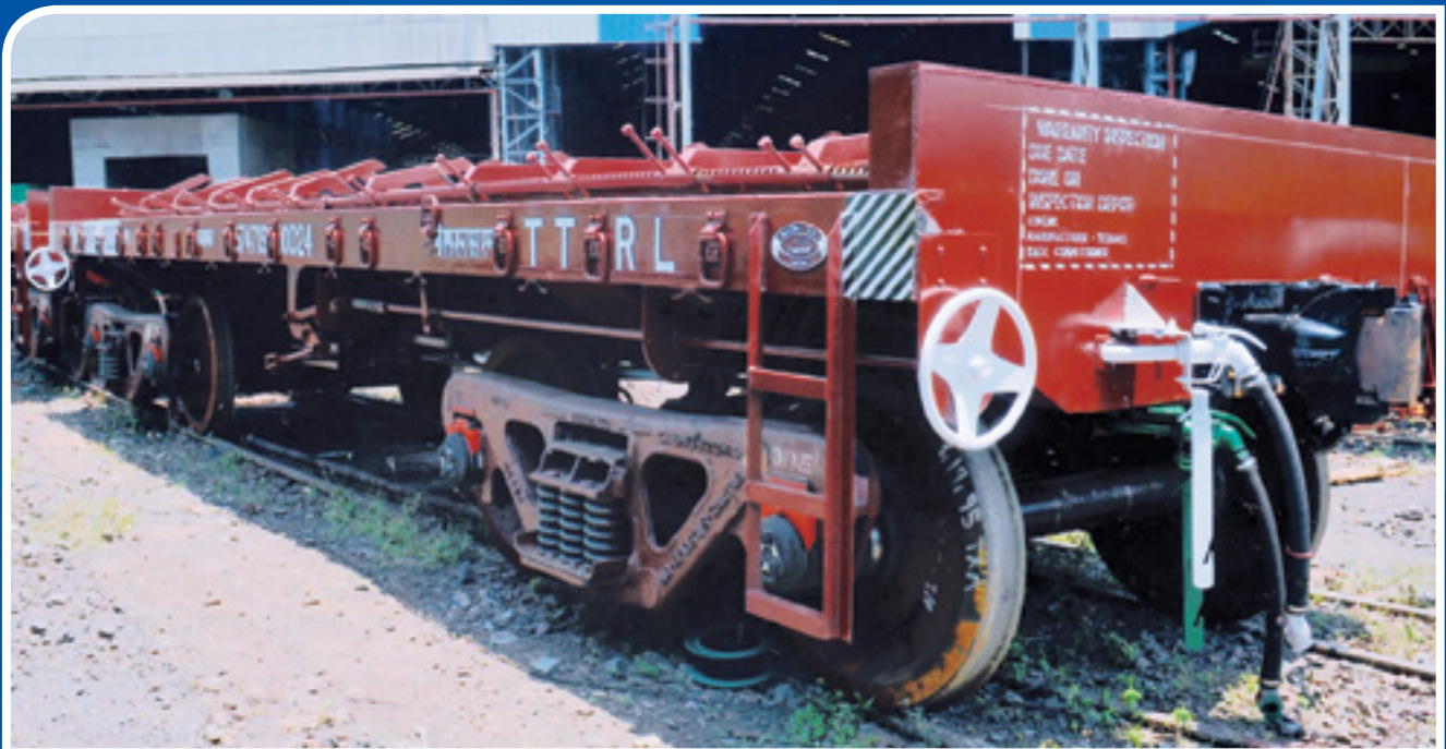
BFNSM Wagon Rake for carrying Steel Coils, manufactured by Texmaco and supplied by Texmaco Touax JV
