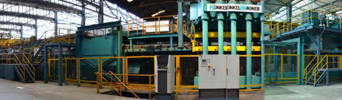
New 2<sup>rd</sup> High Pressure Moulding Line at the Old Foundry
