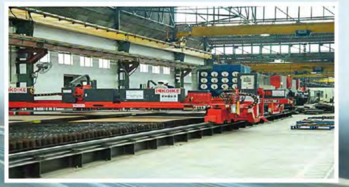
Plasma-Oxy Cutting machine, Koike, Japan
