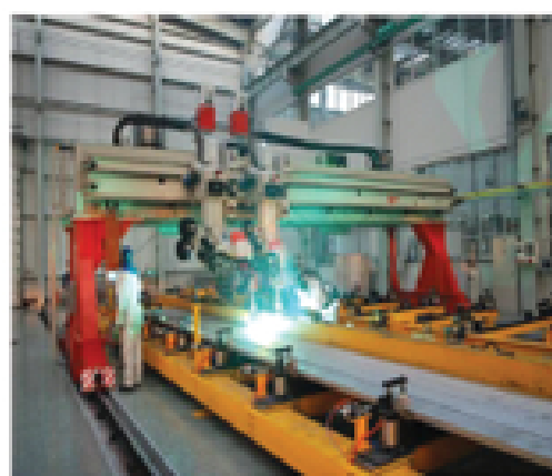
▲ Semi Automated Welding Machine
